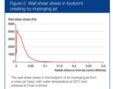
The water from each jet of the rotary jet head creates a moving footprint on the tank walls in the 360-degree indexed cleaning pattern (as mentioned above). Because of the significantly higher impact force of the rotary jet head and subsequent increase in wall shear stress, it is possible to predict the required cleaning time more accurately when using a rotary jet head.
