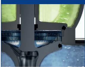
**Seat push:** The lower plug is pushed downwards thus cleaning the plug seal, seat and leakage chamber through CIP flow.
