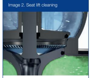
**Seat lift:** The upper valve plug is raised off the seat thus cleaning plug seal, seat and leakage chamber through CIP flow.
